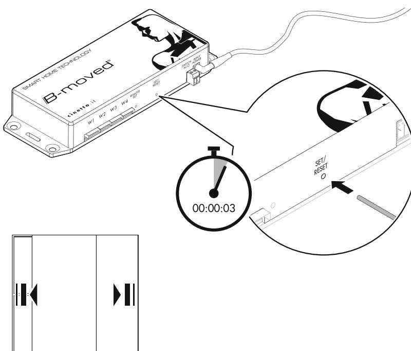
Start the self-learning cycle to make the automatic set-up of the run of the doors pressing at least 3 seconds the "SET / RESET" button on the power unit. All the doors, one by one, starting from the first left door on the wardrobe, will move at reduced speed until their final stoppers.
