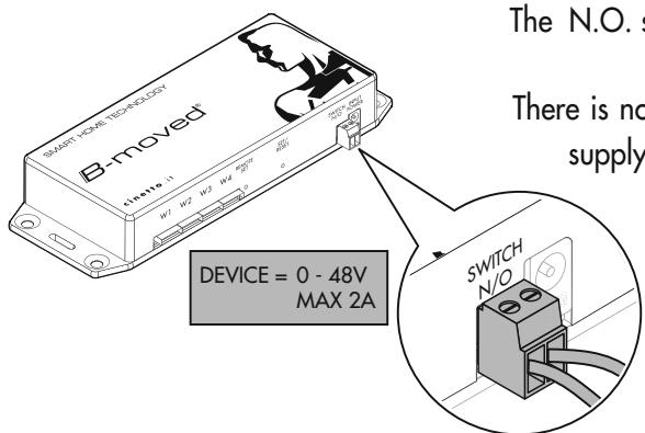
The switch can manage devices with nominal tension between 0 and 48V and a maximum electric current of 2A.
