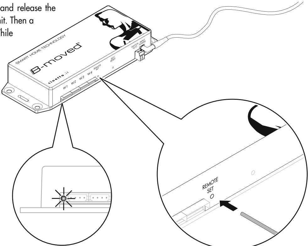
To unpair the remote control unit, press and release the "REMOTE SET" button, after which the red LED will flash. Press the "REMOTE SET" button again and keep it pressed until the led stops flashing. When the button is released, the red LED will flash 5 times to confirm the unpairing.
