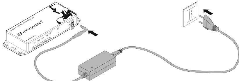
After connecting all the electric motors to the control unit and after closing manually all the doors is possible to connect the control unit to the power supply.
