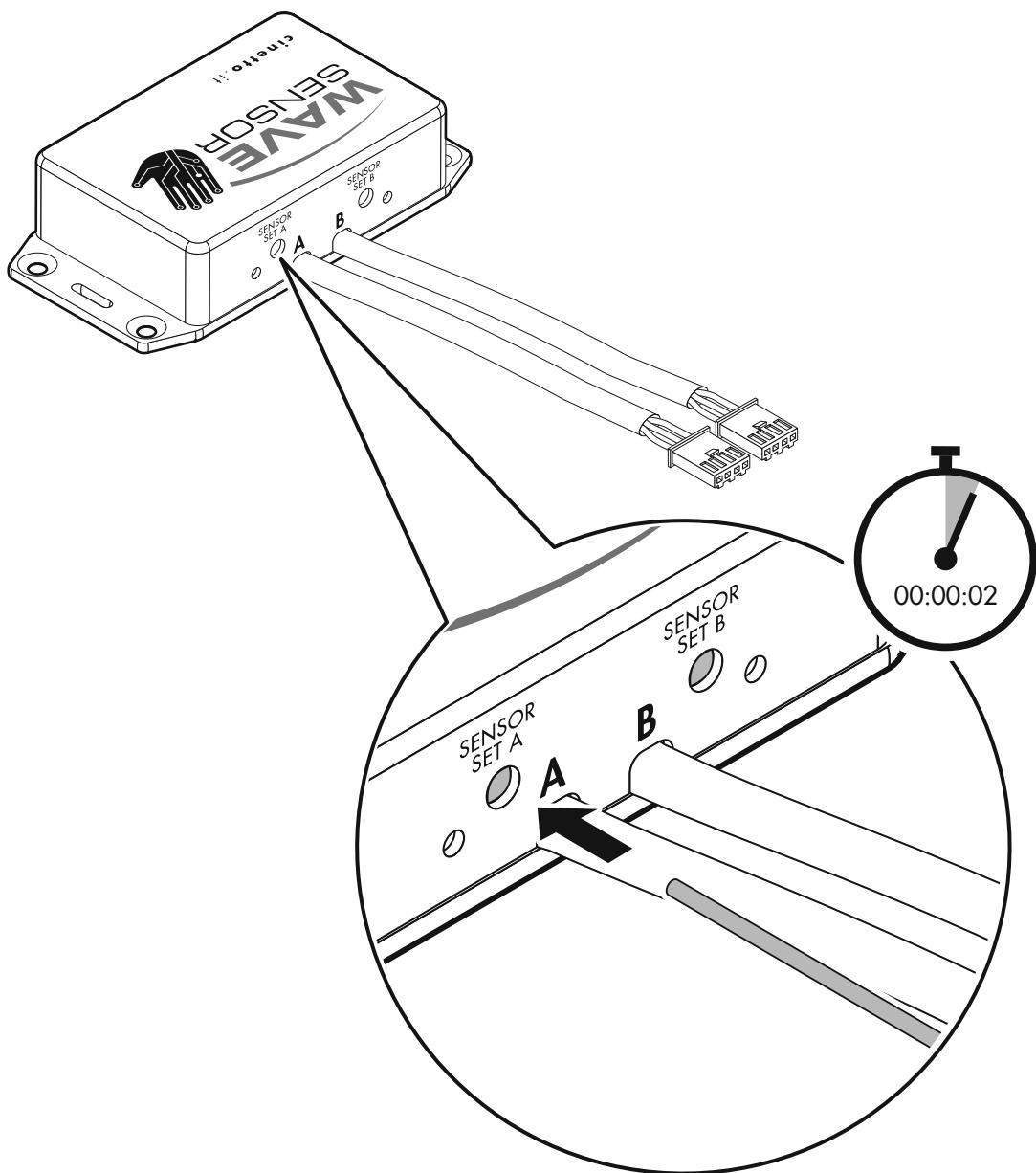
Touch the sensor you want to pair, this will be immediately recognised, causing the LED to flash quickly twice before turning off. At this point the procedure is completed and the devices are correctly paired.
